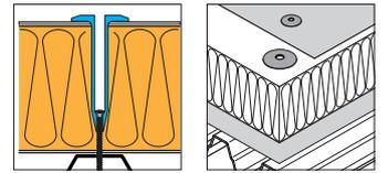
Overlap length between sleeve and fastener: 20 mm
